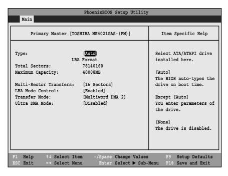
Figure 2. Primary Master Submenu
